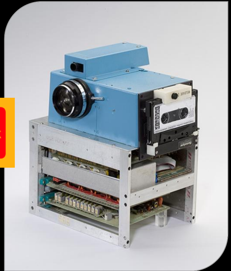
The first digital camera (C.C.D - Charge Coupled Device) created by Sasson in 1975.
